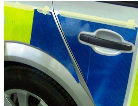
**Step 2.** Remove the liner and squeegee piece into place.
